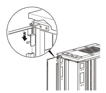
4. Using the included M5 hex wrench, remove the door bumpers at the top and bottom of the door frame.
